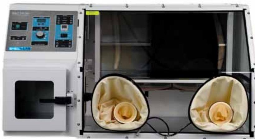
Modular unit with 13.7 cu. ft. work space and a 300-Petri plate capacity
